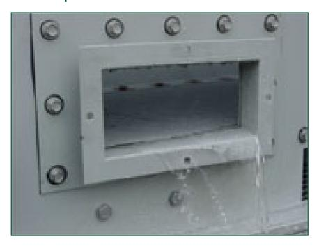
A factory-installed clean out port
