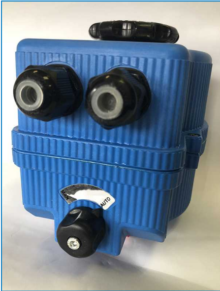
Purge valve actuator position "AUTO"
